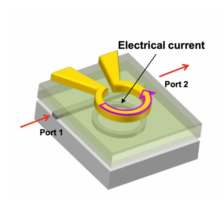
The magneto-optic modular: Gold coil (top), synthetic garnet (green in middle), silicon micro-ring resonator and waveguide (bottom). Port 1 and 2 are the input and output for the optical transmission.
