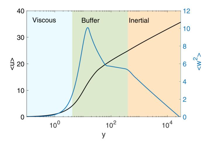
The mean velocity curve (black) and variance (blue) of a fluid in different parts of the boundary layer.
