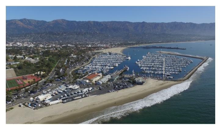
Construction of the Santa Barbara harbor altered the flow of sand along the coast, completely reshaping the area's beaches.
