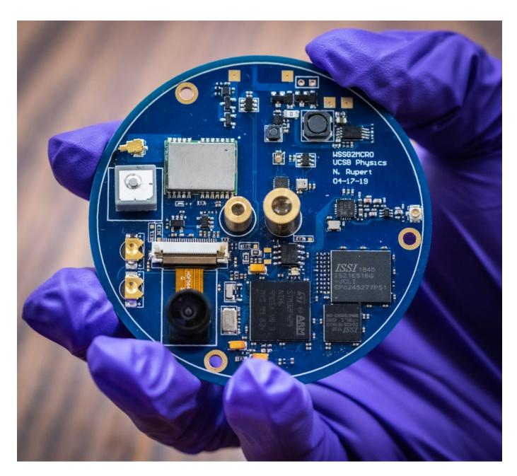
The wafer-scale spacecraft on the flight.
