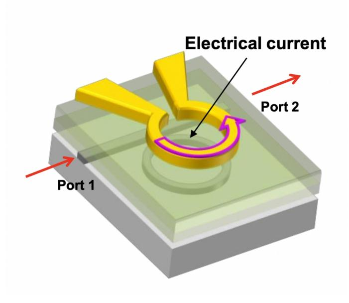
The magneto-optic modular: Gold coil (top), synthetic garnet ( green in middle), silicon micro-ring resonator and waveguide (bottom). Port 1 and 2 are the input and output for the optical transmission.
