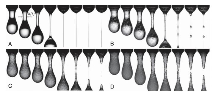
A droplet of silicone oil pinches of from fluids with different concentrations of 140  $\mu$ m particles: (A) is pure liquid, (B) is 2% concentration, (C) is 20%, and (D) is 50%.
